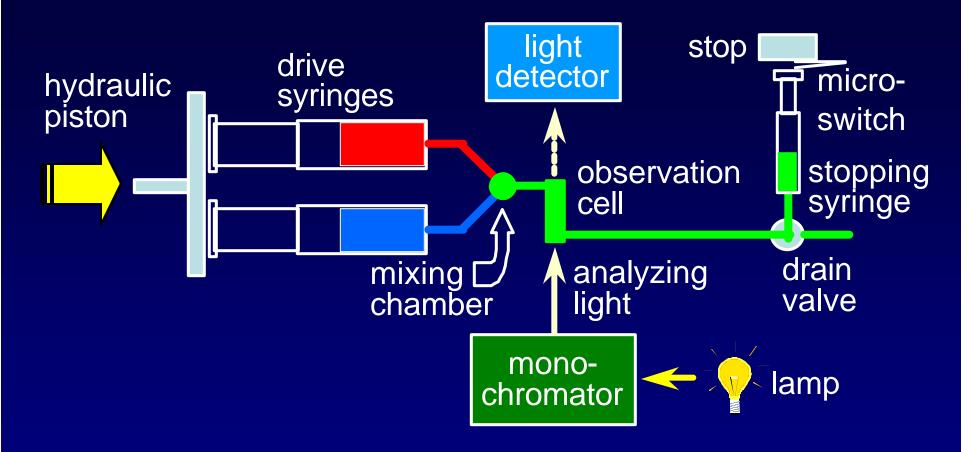
Time resolution limited to about 1 ms by interval between mixing and observation
